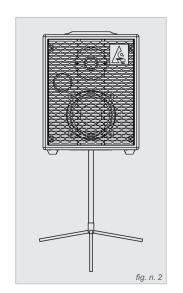
If someone want to use it in vertical position, this amplifier must be positioned in a stand as show in figure n. 2.
