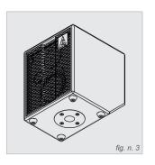
Feet on the bottom of the box are only for avoiding to damage the painting when the user put the amplifier on the ground before put it on stage (figure n. 3).
