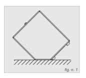
When this amplifier is used on the ground, it must be used as show in figure n. 1.
