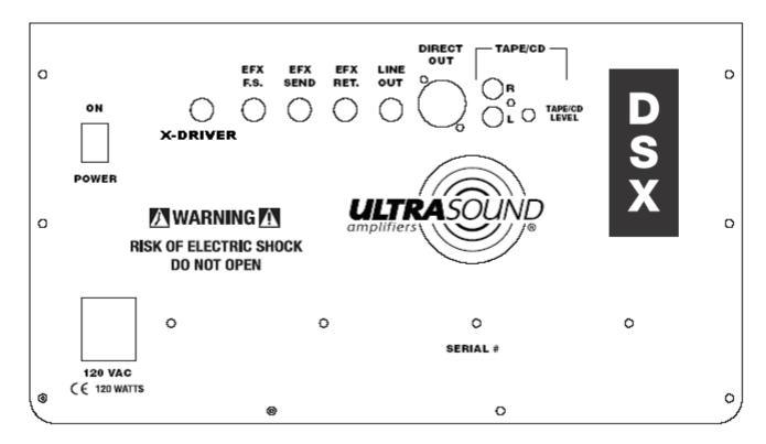
**X-DRIVER:** This jack is for connection to a non-powered extension speaker like the **Ultrasound XTC**. This jack provides a "speaker level" signal. The minimum load that can be driven is 4 ohms.
