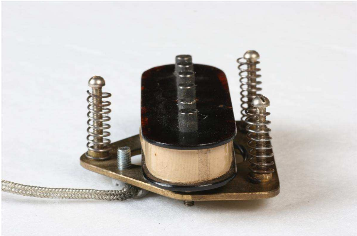
Photo 04-2. Single coil pickup, similar (bobbin, 6 cylindrical magnets) to those found on Gibson lap-steels between 1951 and 1956 and on Rio lap-steels, but with a higher resistance (9.52 k \Omega , vs. ca. 8k \Omega on Gibsons). Set with 3 screws, in a triangle layout, allowing height adjustment. Metal plate craftsmanship is at Switzerland's best level. Courtesy of the Musée des Musiques Populaires.
