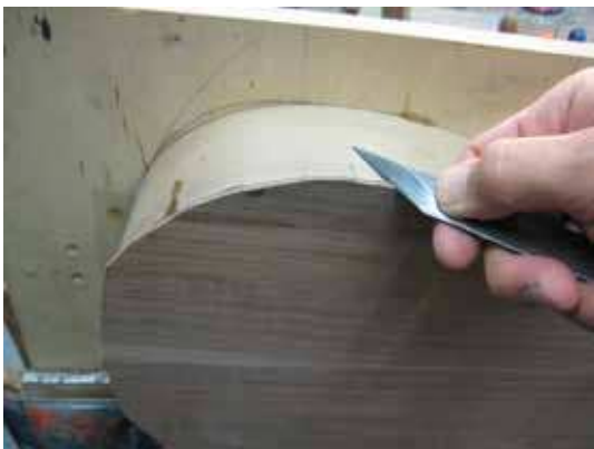
Trimming the edges
