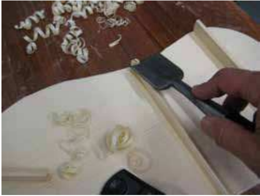
Shaping of the transverse bars
