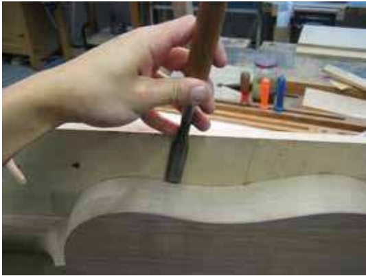
Releasing the body from the plate
