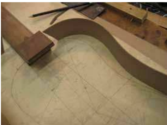
Sides before and after gluing
