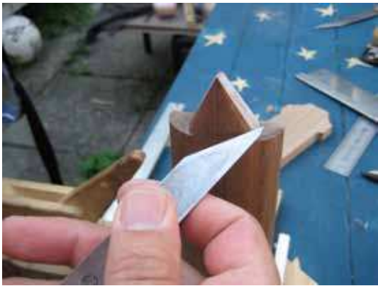
Cutting of the V-joint
