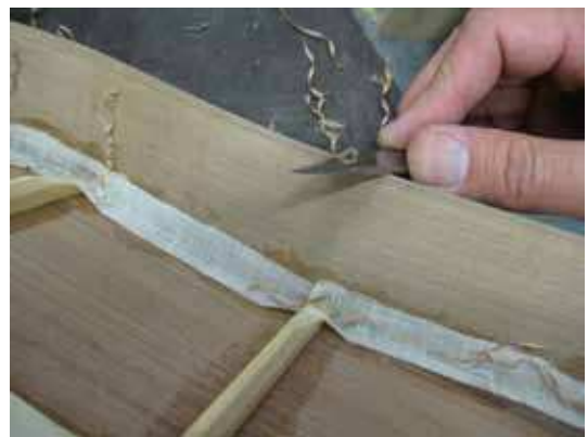
marking and cutting a curvature on the plane of the soundboard, designed to add clearance to the strings
