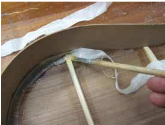
reinforcing the joints with linen and parchment
