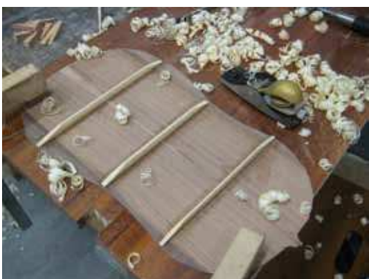
Trimming and shaping the transverse bars
