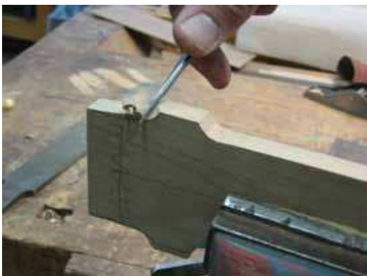
Shaping of the headstock
