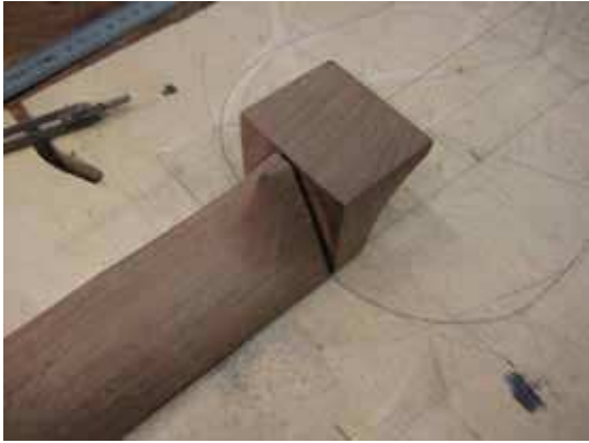
Neck attached to board, and bending of first rib
