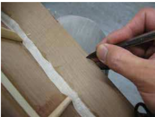
marking and cutting a curvature on the plane of the soundboard, designed to add clearance to the strings
