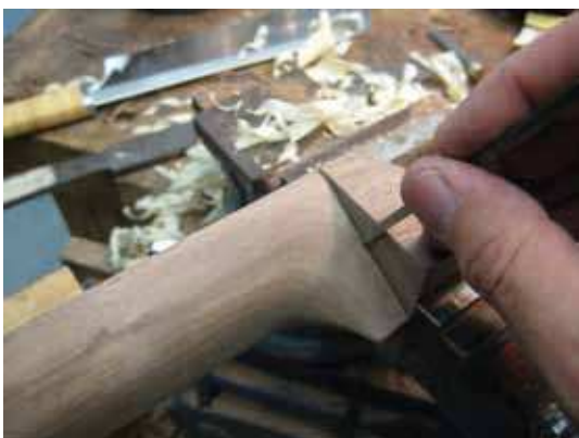
Cutting of the groove
