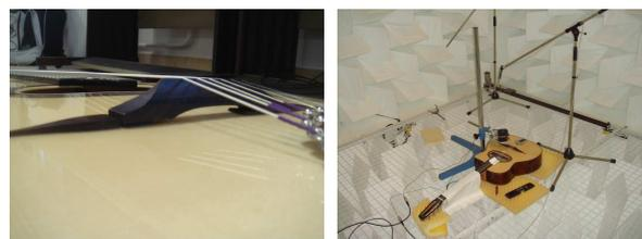
(a) close-up view of the gypsy guitar-bridge. (b) An image of the shaker, microphone and guitar setup in the anechoic chamber.
