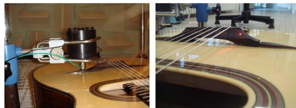
(c) A close-up of the shaker at the bridge in the anechoic chamber (d) A close-up of the Vibrometer's laser on the guitar bridge.
